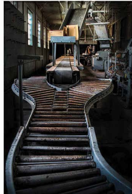
Bottling line split, T. W. Samuels Distillery, Deatsville. The split lines might convey boxes on one side and bottles on the other, which then come together efficiently.
